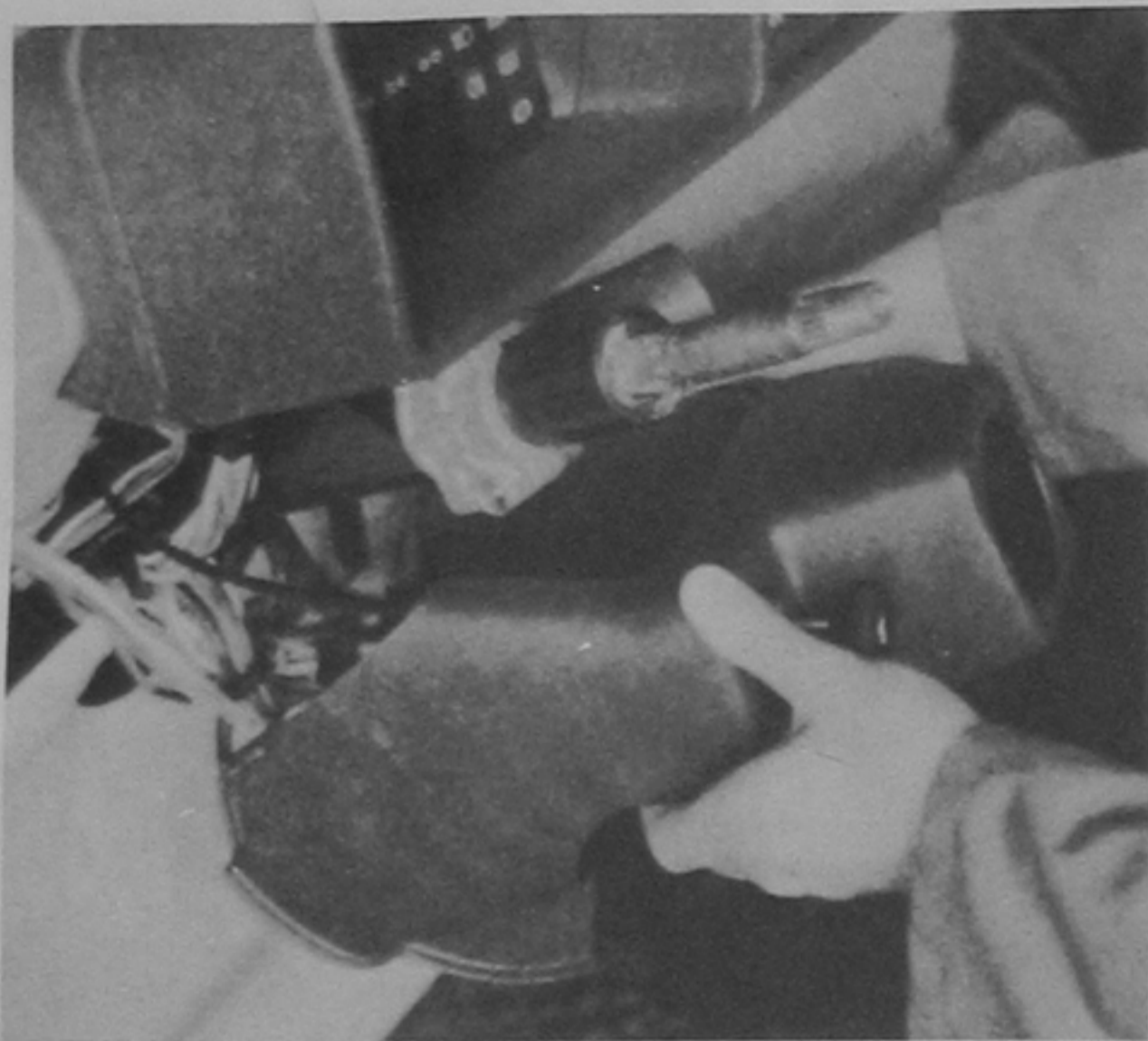
Fig. 10.3 Withdrawing steering column shroud (Sec 6)
